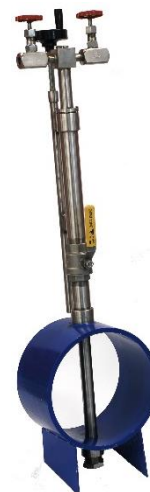
Multipoint Pitot Tube for liquid and gas can be used to calculate flow in larger ducts or in areas of turbulent flow.
